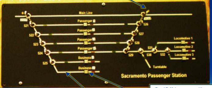
On/Off buttons-if red LED is on, track is on
